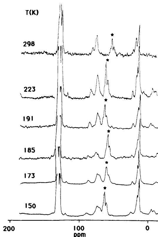
Figure 3. 50.3-MHz 13 C CPMAS NMR spectra of α-MC recorded at different temperatures. Other spectral parameters are as in Figure 2.
